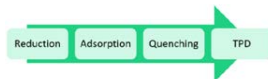
Figure 3: Experimental procedure for investigating the amount of nitrogen adsorbed on the surface of an iron-based catalyst.
