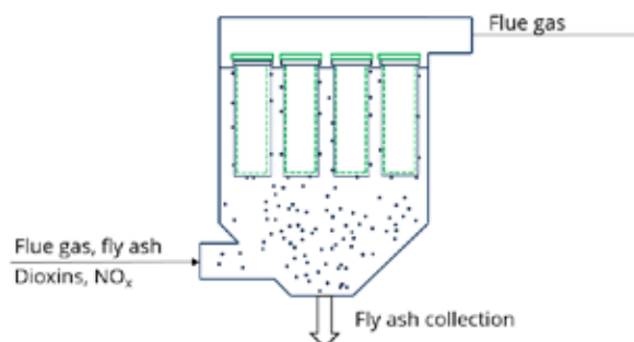
Figure 2: Catalytic filter bag design, removing fly ash, dioxins and NO x in a single process step.
