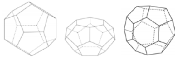
Figure 1: Schematics of the cavity structures in the natural gas hydrate. From left is the common small 5 12 cavity and then the large s1 5 12 6 2 cavity. Right is the large s2 cavity.
