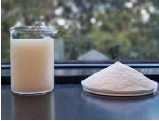
Figure 1: An acrylic dispersion (on the left side) and its powder form produced by the spray drying process at the CoaST DTU Chemical Engineering Laboratory.
