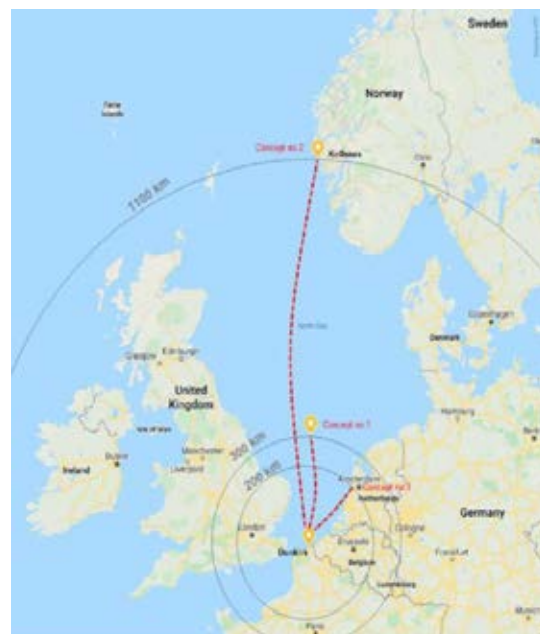
Figure 1: Carbon dioxide transport concepts for the Dunkirk 3D Project.
