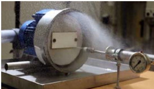
Figure 2: The pulsating water jet erosion tester in CoaST.
