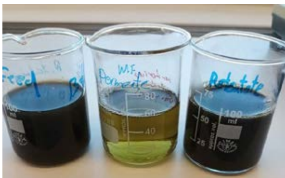
Figure 1: Feed, permeate, and retentate after the microfiltration process.
