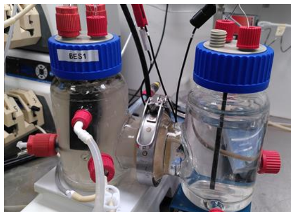
Figure 3: First BES tested in the project, converting CO 2 into acetic and butyric acid.
