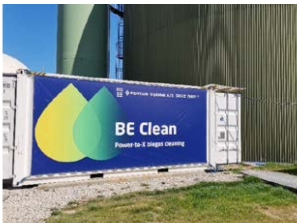
Figure 1: The mobile test unit used for pilot scale tests at a biogas plant near Slagelse
