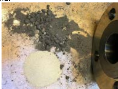
Figure 2: Agglomerates from defluidization compared to fresh sand.
