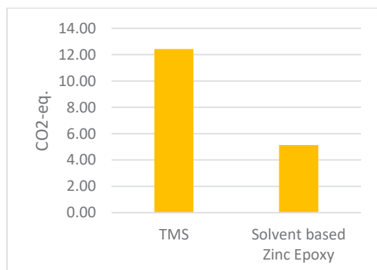
Figure 2: Global warming contribution from two alternative coating systems - one using TMS as primer coat - the other use zinc epoxy.
