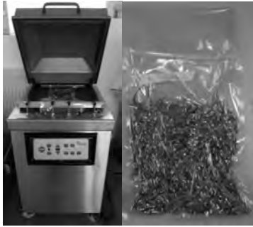
Figure 2: Left: Vacuum packaging machine, Variovac EK10. Right: Grass silage bag
