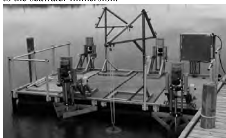
Figure 2: Cylindrical seawater test setup.
