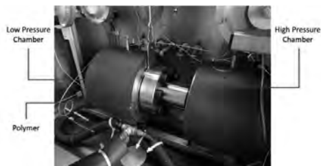
Figure 3: 2-D permeation cell assembled prior to a run [3].
