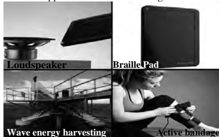
Figure 1: Different applications of DEAP, such as thin lightweight loudspeakers, e-books for blind people, wave energy harvesters and bandages to increase the blood circulation and ease the recovery e.g. after surgeries.
