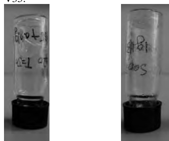
Figure 5a (left), 5b (right). Reactivity of PMMA/HMS-301 microcapsules in V35 and catalyst at 50 ^\circ\text{C} (left) and 120 ^\circ\text{C} (right)
