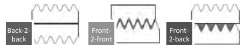
Figure 2: The different configurations for the adhesion of the films. The back-2-back configuration is where the flat sides are adhered together. The corrugated sides are adhered together in the front-2-front configuration and for the front-2-back configuration, a corrugated side is adhered with a flat side.
