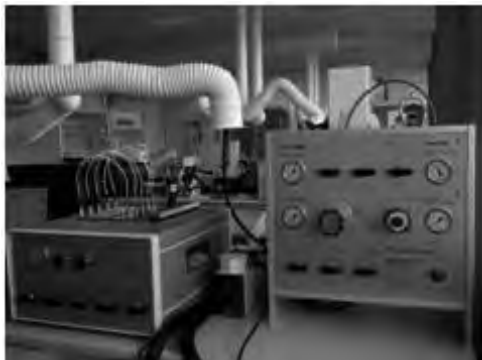
Figure 3: Rocking Cells produced by PSL Systemtechnik. The picture shows the Rocking Cells setup consisting of the cooling bath with 5 test cells and the high pressure panel.
