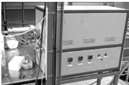
Figure 2: Photograph of oven with controlled gas composition.
