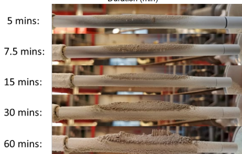
Figure 3: Effect of experiment duration on deposit formation rate. Experiments were conducted with cement bypass dust, with a furnace temperature of 1400°C, flue gas temperature 1099°C, gas velocity 2.7 m/s, probe surface temperature 550°C, feeding rate of 100g/h.
