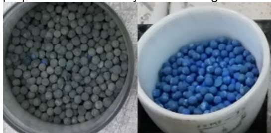
Figure 21: Two Co-Sn/Al 2 O 3 catalysts with the same amount of Co and Sn but with slightly different preparation methods. Left: method 1. Right: method 2.
