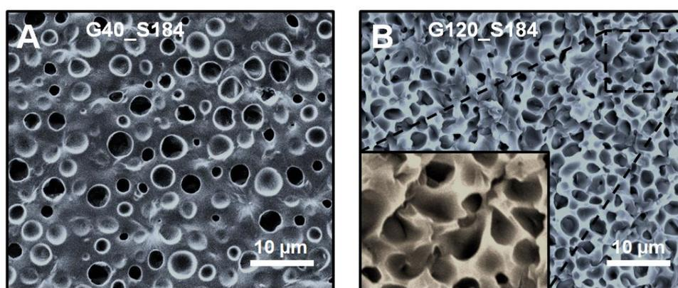
**Figure 1.** SEM images of composites representing discrete glycerol droplet morphology (A) and bicontinuous morphology (B) with interconnections present between the adjacent glycerol domains as illustrated in the enlarged picture in inset.
