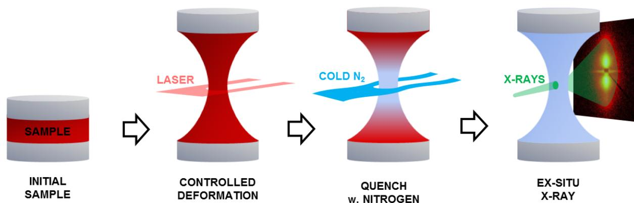
Figure 1: Experimental protocol for studying the correlation between extensional rheology and final morphology of polymeric fibers.
