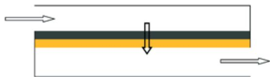
**Figure 5:** The concept of a catalyzed filter: The flow through the filter is forced across a catalyzed filter wall (yellow) while the soot in the exhaust gas becomes entrained in the inlet channel, forming a layer (grey).
