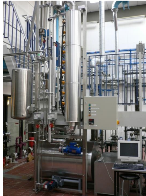
Continuous distillation in bubble-cap tray column
