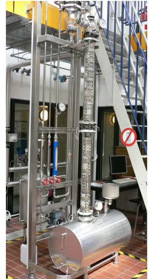
Batch distillation of alcohols using structured packing
