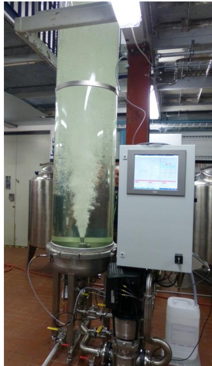
Fixed bed for immobilized enzyme processes, ion exchange or chromatographic separations
