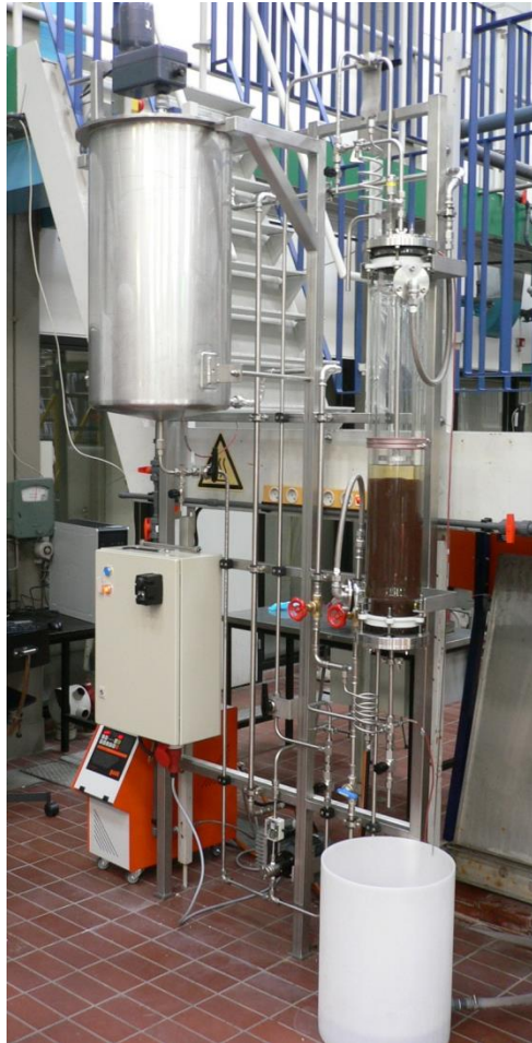
Fixed bed for immobilized enzyme processes, ion exchange or chromatographic separations
