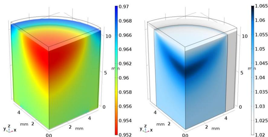
**Figure 1:** Simulation results from a simulation of a stack of 450 dielectric elastomers. The electrodes are applied in the middle of the stack covering 64% of the total area. The picture to the left displays the stretch ratio in the z-direction, and the ratio of the normalized electric field to the initial electric field is displayed on the picture to the right.
