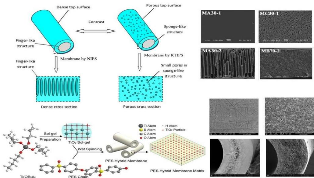
**Figure 1:** The contrast of the membranes prepared by NIPS and RTIPS method; SEM micrographs of PES membranes and PES/TiO<sub>2</sub> hybrid membranes
