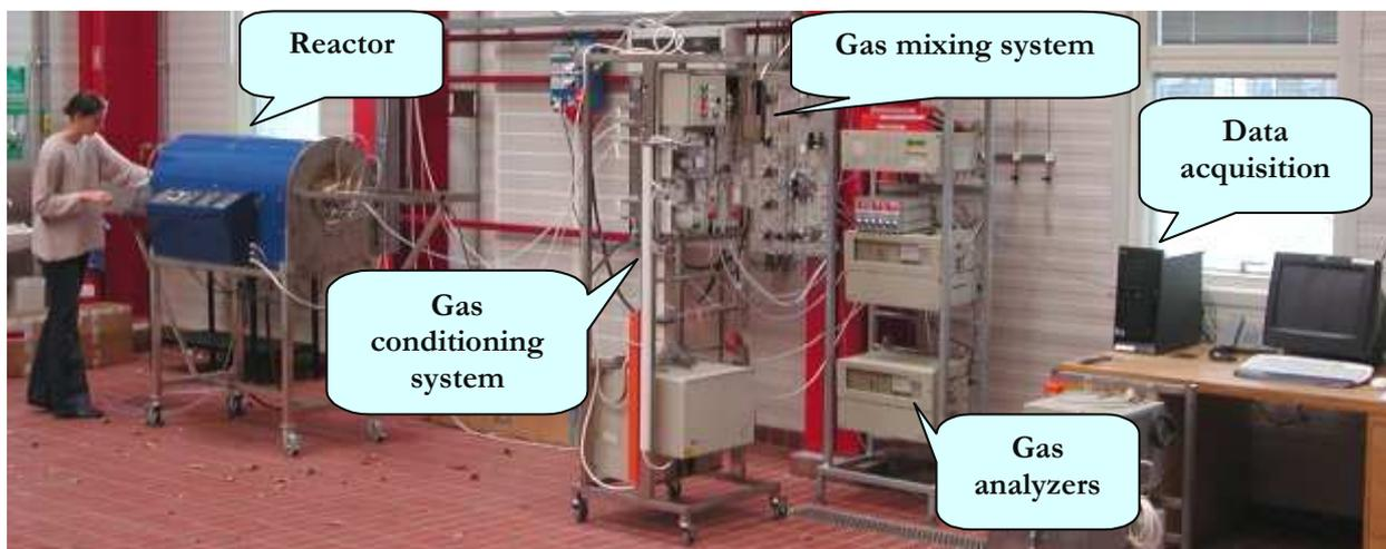
**Figure 3:** Experimental set-up for studying the release of inorganic elements from a burning wood sample.
