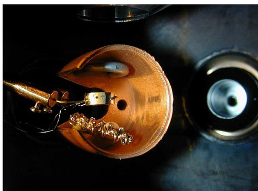
**Figure 2:** Inside the UHV chamber. The ruthenium single crystal is seen in the center of the copper house. A tungsten wire wrapped with gold for evaporating Au onto the surface of Ru, is seen under the crystal.
