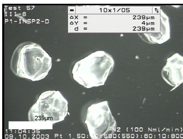
**Figure 4:** 2wt.% Na-alginate caught in 2wt.% CaCl<sub>2</sub> solution and dried in a Petri dish. JetCutter settings: Rotational speed of cutting wires: 4000rpm; Flowrate through nozzle: 0.3g/s; Nozzle diameter: 200µm.
