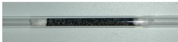
**Figure 3:** A catalytically tested 2wt% Ru/spinel for the dehydrogenation of ethane. The catalyst is placed in a quartz tube reactor with quartz wool plugs at the ends of the catalyst.
