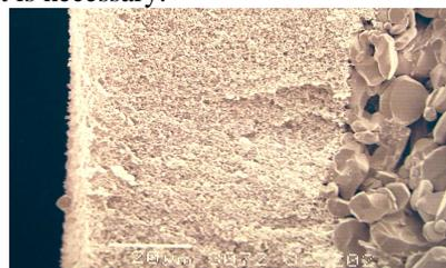
**Figure 3:** A SEM picture of a  $\text{MgO}$  membrane. The coarse substrate structure is seen to the right.
