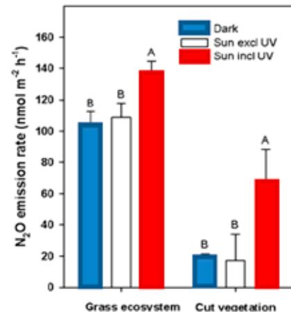
Field measurements of  $N_2O$  emissions in a Danish grassland. Grass ecosystem = intact soil and plants. Cut vegetation = cut vegetation shoots isolated from soil with a membrane. Dark simulates the hitherto  $N_2O$  measurement in ecosystems, Sun excl UV = PAR (90%) transparent ecosystem chamber & Sun incl UV = PAR (90%) and UV (83%) transparent ecosystem chamber (Bruhn et al., 2014b).
