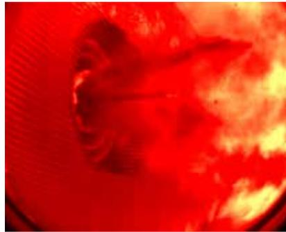
Thermal image of pulverised wood flame in the power plant of Høfor. The dark structures are wood particles leaving the burner. Probe for measurement of temperature and gas composition is inserted through the centre of burner.
