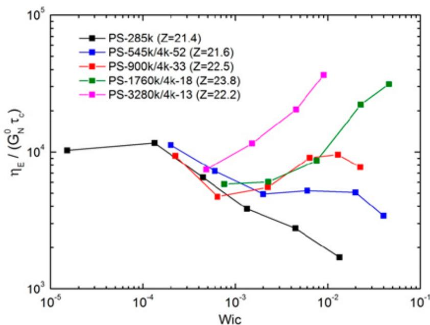
The figure shows the normalized extensional viscosity as a function of the normalized stretch rate for five polystyrene solutions. The solutions contain different concentrations of polystyrenes from 10% (pink curve) to 100% (black curve). The figure reveals that the nonlinear rheological behavior of polymer chains is not universal but concentration dependent.
