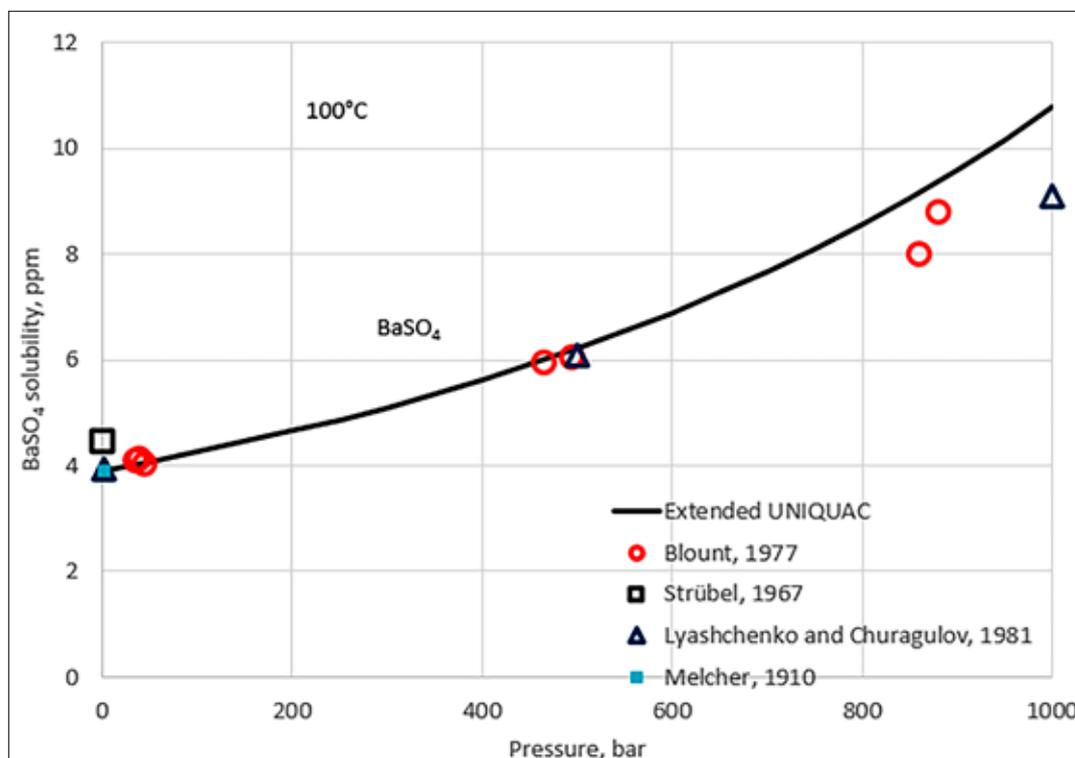
The figure shows the solubility of BaSO<sub>4</sub> (barite) at 100°C as a function of pressure from 1 to 1000 bars. Experimental data from various sources are plotted together with the curve calculated with the Extended UNIQUAC model.
