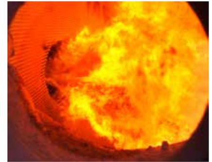
Video image of pulverised wood flame in the power plant of Høfor. Flame light from soot particles at burner exit indicated ignition. The measurements were done in collaboration with Johan Wadenbäck.
