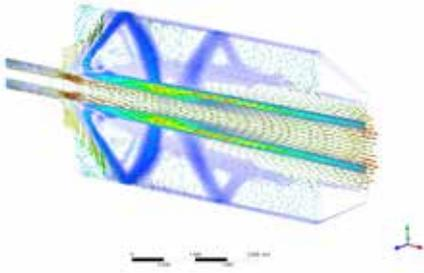
Full-scale CFD modelling of a 30 MW bio-dust flame: Velocity field and fluid and combustion of bio-dust.
