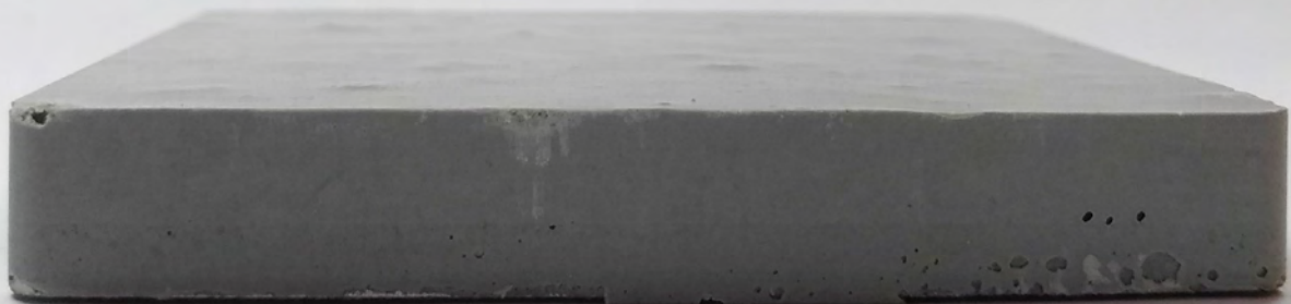
A hydrocarbon intumescent coating with a thickness of 6 mm applied on the surface of a grit-blasted steel plate. The coating is a two-component (base and curing part) epoxy-based system which is targeted specifically at passive fire protection against hydrocarbon fire scenarios.
