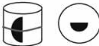
Figure 3: The left side shows a clinker which is embedded vertically in epoxy and the sample is cut along the line. The right side shows a top view of the sample which has been cut in half. This sample is studied by an optical microscope.
