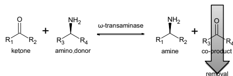
Figure 1. Simplified general scheme of \omega -transaminase reaction and equilibrium shift strategy of co-product removal
