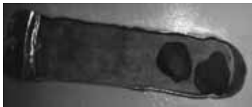
Figure 2: Two clinker half. One where ash is added and the other one is kept as a reference.
