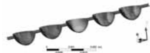
Figure 1: Schematic representation of the designed microreactor. Due to the existence of two symmetry planes ( xz and xy planes), only a quarter of the reactor was simulated and is illustrated.
