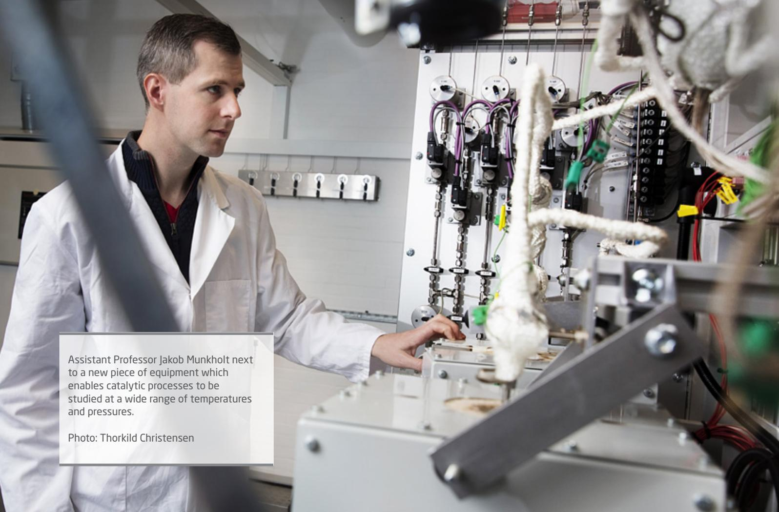
Assistant Professor Jakob Munkholt next to a new piece of equipment which enables catalytic processes to be studied at a wide range of temperatures and pressures.
