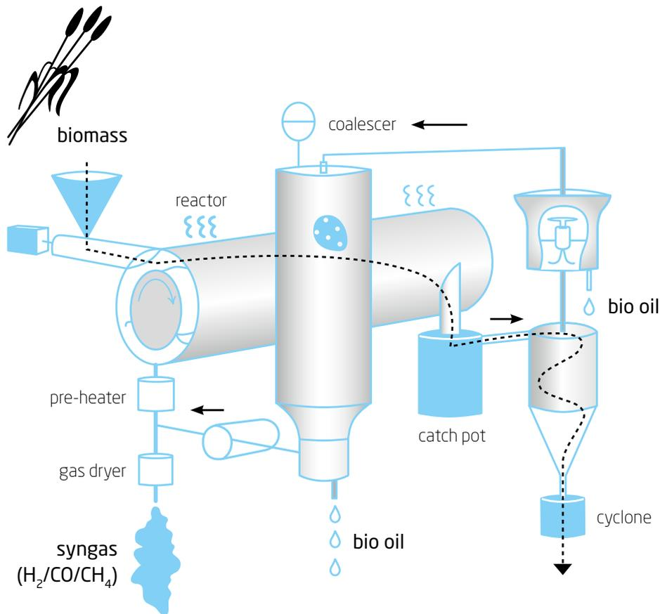
The Pyrolysis Centrifuge Reactor (PCR) used in Norazana Ibrahim's research converts biomass into bio-oil, gas and bio-char. Straw is introduced by the screw feeder into the centrifuge reactor. A cyclone is used for char collection, and a condenser and a coalescer is used for bio-oil collection. A pump re-circulates a part of the formed gas.
