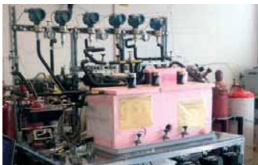
**Figure 2:** High pressure crystallizer setup.
