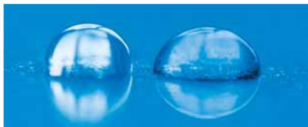
**Figure 1:** Water droplet on a hydrophobic surface to the left and on a hydrophilic surface to the right.
