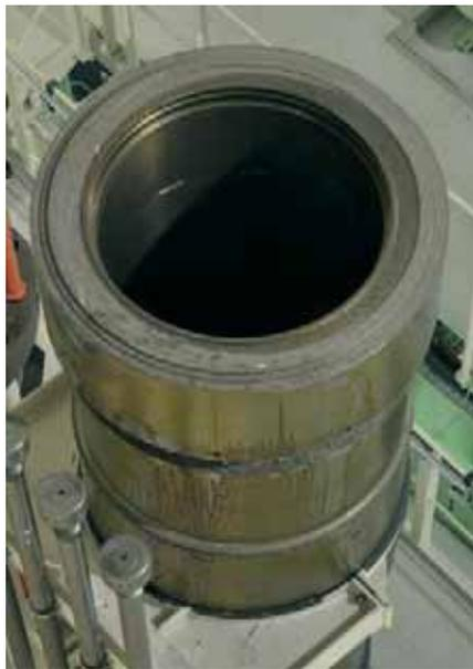
**Figure 2:** View of a large ships engine cylinder at the container ship, Matz Maersk. The internal liner surface is exposed to corrosive flue gas components, wear from piston movements as well as high temperatures and pressures.
