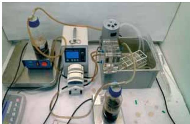
**Figure 1:** Off-line testing of wheat straw hydrolysate.
