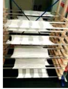
**Figure 1:** The device used to pre-stretch the thin filled PDMS elastomer films. The pre-strains were adjusted by changing the position of the metal rods.
