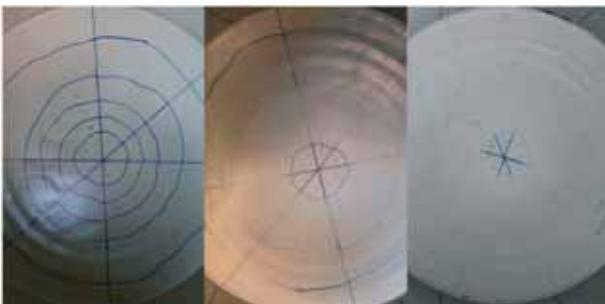
**Figure 3:** Circular erosion pattern observed on can bottom. 0h (left), 34h (middle) and 180h (right) exposure time.
