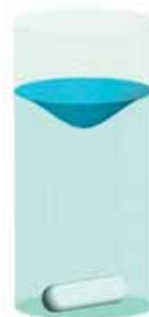
**Figure 2.** The magnetically stirred reactor filled with 8 ml liquid.
