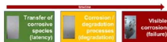
Figure 1: Degradation of protective organic coating through accelerated exposure test (neutral salt spray test ASTM B-117) – An example
