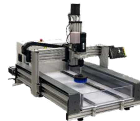
Figure 1: Automated underwater cleaning system (AUCS) for laboratory scale simulation of underwater rotary brush cleaning
