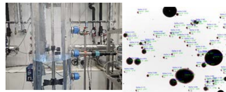
Figure 2: Use of Shadowscope in the reactor and an example of an analysed bubble image.
