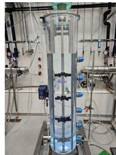
Figure 1: Pilot scale reactor, with a working volume of 180 L. Equipped with standard ring larger, Rushton turbines, and baffles.
