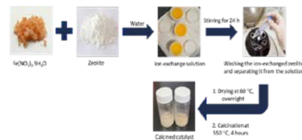
Figure 1. Representative synthesis process (ion-exchange) for fabricating Fe-zeolite catalyst.
