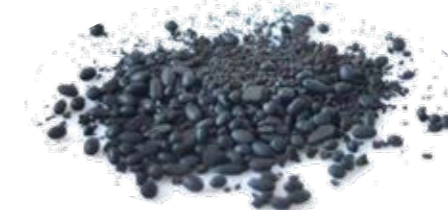
Figure 3: Sample of the crushed catalyst pellets after processing for 90+ hours.
