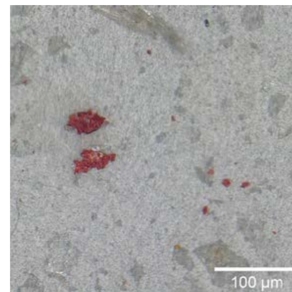
Figure 1: Light microscope image of some microplastics from antifouling coatings released during controlled exposure.
