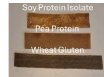
Figure 2: Extruded films of soy protein isolate, pea protein and wheat gluten.
