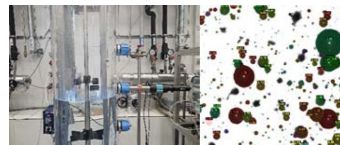
Figure 2: Use of ParticleSight in the reactor and an example of an analysed bubble image.
