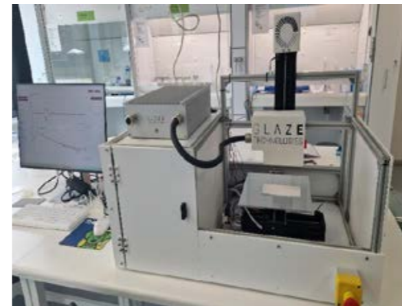
Figure 43: Terahertz cross-correlation spectroscopy and imaging system used in this study in reflection mode for coating characterization.
