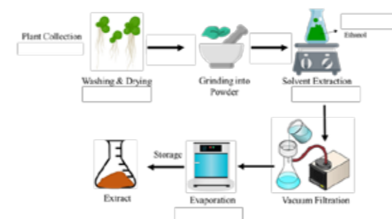
Figure 1. Schematic representation of the extraction process of bioactive compounds from aquatic plant biomass.
