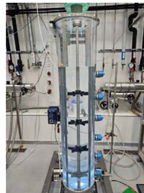
Figure 50: Pilot scale reactor, with a working volume of 180 L. Equipped with standard ring sparger, Rushton turbines, and baffles.
