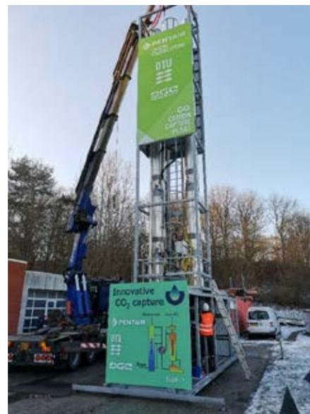
**Figure 1:** The newly constructed mobile test unit for biogas upgrading raised at Mølleåværket A/S.
