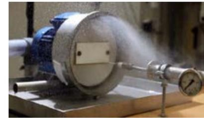
**Figure 2:** The pulsating water jet tester in CoaST.
