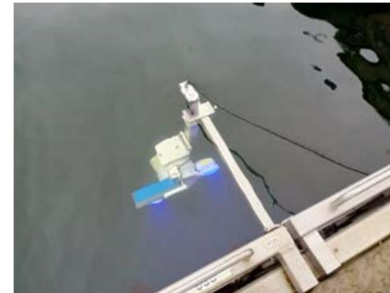
**Figure 3:** Long term underwater camera mounted on the CoaST raft at Hundested with different colored LEDs, a fluorescence filter, and a servo motor wiper to prevent fouling accumulation.
