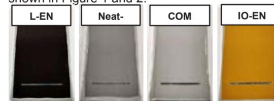
**Figure 1:** Samples prior to salt spray exposure test.
