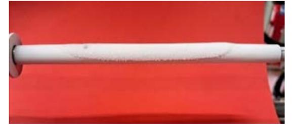
**Figure 2:** Deposition layer on deposition probe.
