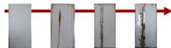
**Figure 1:** Degradation of protective organic coating through accelerated exposure test (neutral salt spray test ASTM B-117) – An example
