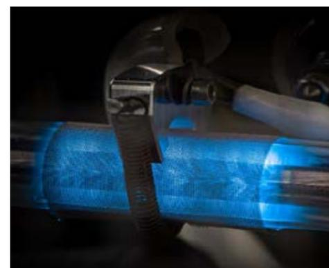
**Figure 1:** Ignited Ar plasma seen in filamentary mode generated in a cylindrical DBD in the experimental plasma reactor at DTU in the department of Chemical and Biochemical Engineering.
