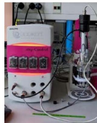
**Figure 1:** Set-up of the 250ml applicon reactor, in which the experiments are being executed.
