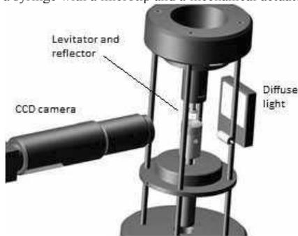
**Figure 1:** Illustration of the levitator setup. The horn and reflector are enclosed in a chamber which is not shown in the figure.
