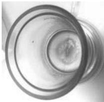
**Figure 2:** Formation of gel layer on the membrane surface reduces the permeate flux
