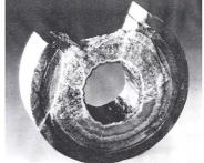
**Figure 1:** CaCO<sub>3</sub> Deposition in Tubing [2]
