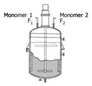
Figure 5: The emulsion copolymerization reactor.
