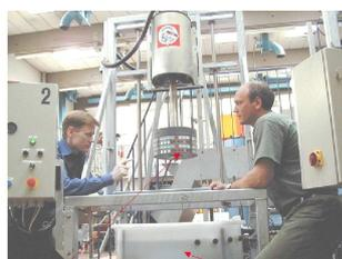
Rotor with paint samples Tank of artificial seawater
