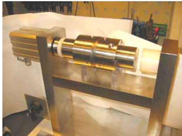
**Figure 2:** Photograph of the test fuel cell
