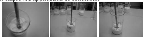
**Figure 5:**  $\alpha$ -cellulose with 30%, 40% and 50% dry matter, note embedded impellers
