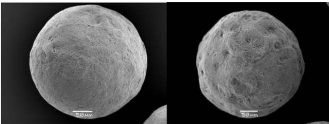
**Figure 4.** Effect of relative and actual average droplet size on coating layer morphology. Left) Coated glass ballotini core from scaling experiment B. Right) Coated glass ballotini core from scaling experiment F.
