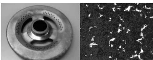
**Figure 3:** Black deposit collected on the burner
