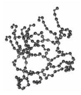
**Fig.2** Schematic view of a reversible network formed by supermolecular interactions. Blue represents the mixtures of two-functional ended amide and red represents the mixtures of three functional ended amide. Dots represent the H-bonds.
