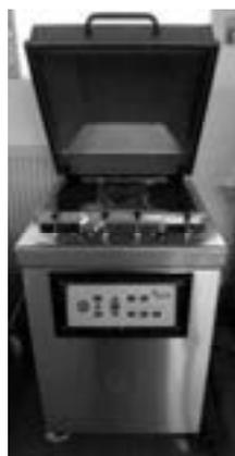
**Figure 1:** Vacuum packaging machine, Variovac EK10
