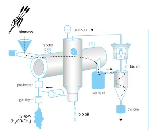
The Pyrolysis Centrifuge Reactor (PCR) used in Norazana Ibrahim's research converts biomass into bio-oil, gas and biochar. Straw is introduced by the screw feeder into the centrifuge reactor. A cyclone is used for char collection, and a condenser and a coalescer is used for bio-oil collection. A pump re-circulates a part of the formed gas.
