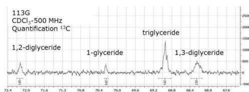
**Figure 2:** Quantified  $^{13}\text{C}$ -NMR spectrum of the biobased one-pot enzymatic alkyd
