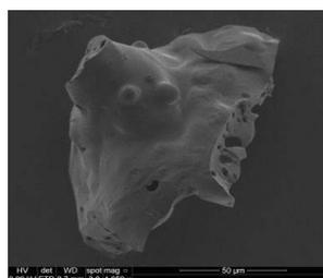
**Figure 8:** SEM image of a molten pinewood particle
