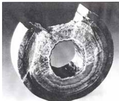
Figure 1.  $\text{CaCO}_3$  deposition in tubing [2]
