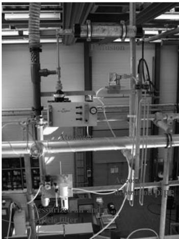
**Figure 4:** Experimental setup for measuring deposition of submicron particles in a 3m long electro polished pipe with a diameter of 6mm.
