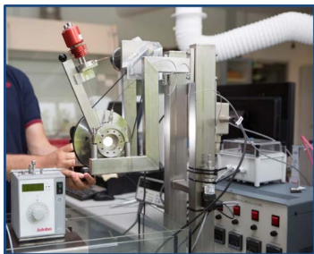
Figure 2: Three-phase VLE cell located at DTU.
