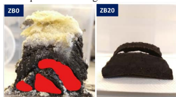
Figure 3: The cross-section of the char ZB0 and ZB20 with the big voids (width >5 mm) highlighted in red.
