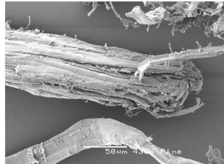
Figure 2: SEM picture of a pine particle.
