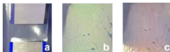
Figure 4: Images of a PDMS-SiO 2 (169 nm) film at various elongations under dark conditions. (a) The film at 0 elongation; (b) the film at 110% elongation; (c) the film at 55% elongation.
