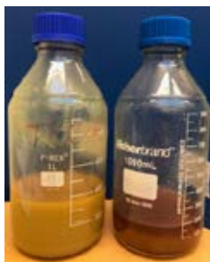
Figure 1: Left) Wax obtained from thermal pyrolysis. Right) Liquid/wax obtained from catalytic pyrolysis.
