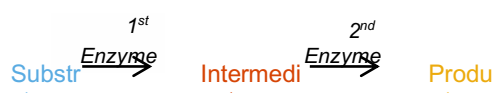
Figure 1: Linear cascade system with two enzymes for sequential reaction without intermediate separation.
