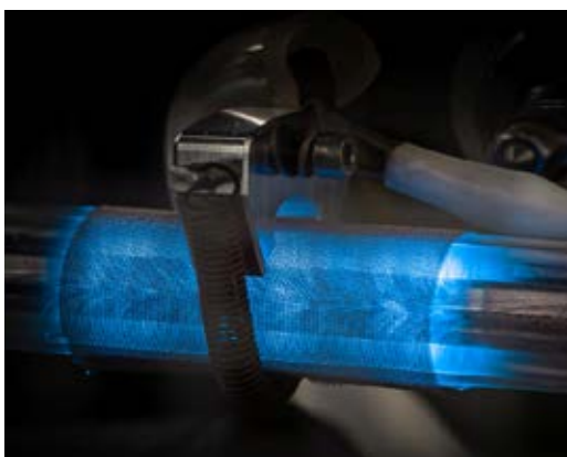
Figure 1: Ignited Ar plasma seen in filamentary mode generated in a cylindrical DBD in the experimental plasma at DTU in the department of Chemical and Biochemical Engineering.
