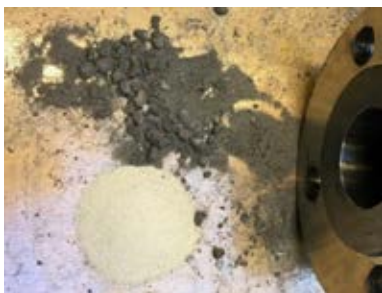
Figure 2: Agglomerates from defluidization compared to fresh sand.
