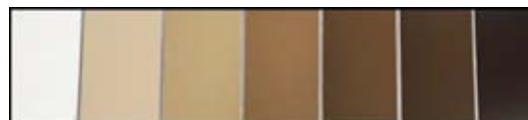
Figure 2: Solventborne epoxy coatings substituting different amounts of lignin from 0 wt.% (left) to 35 wt.% (right).
