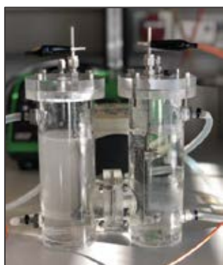
Figure 1: Overview of the lab scale electrolytic cell used for the system characterization.
