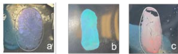
Figure 1: Images of different sized SiO 2 PCs film at various conditions. (a) TEOS: EtOH=1:25; (b) TEOS: EtOH=1:20; (c) TEOS: EtOH=1:15.
