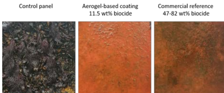
Figure 2: Panels after 6 months of exposure at CoaST Maritime Test Centre. The performance of an aerogel-based coating (middle) is compared to a non-coated control panel (left) and a commercial coating (right). The total concentration of biocidal compounds on a weight basis is indicated.
