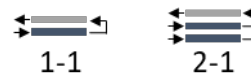
Figure 4: Comparison of different two-stage stage filter designs with serial and mixed cassette configurations. The mixed 2-1 design results in a 29% higher VCF and a 17% lower TMP under the investigated operating conditions.
