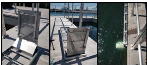
Figure 2: Images of the developed horizontal exposure setup with mounted glass panels for exposure, two on each side. The image to the right shows how the setup is exposed.
