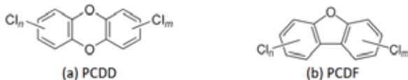
Figure 1: Illustration of chemical structure of dioxins, which is a term describing both (a) Polychlorinated dibenzodioxins and (b) Polychlorinated dibenzofurans.
