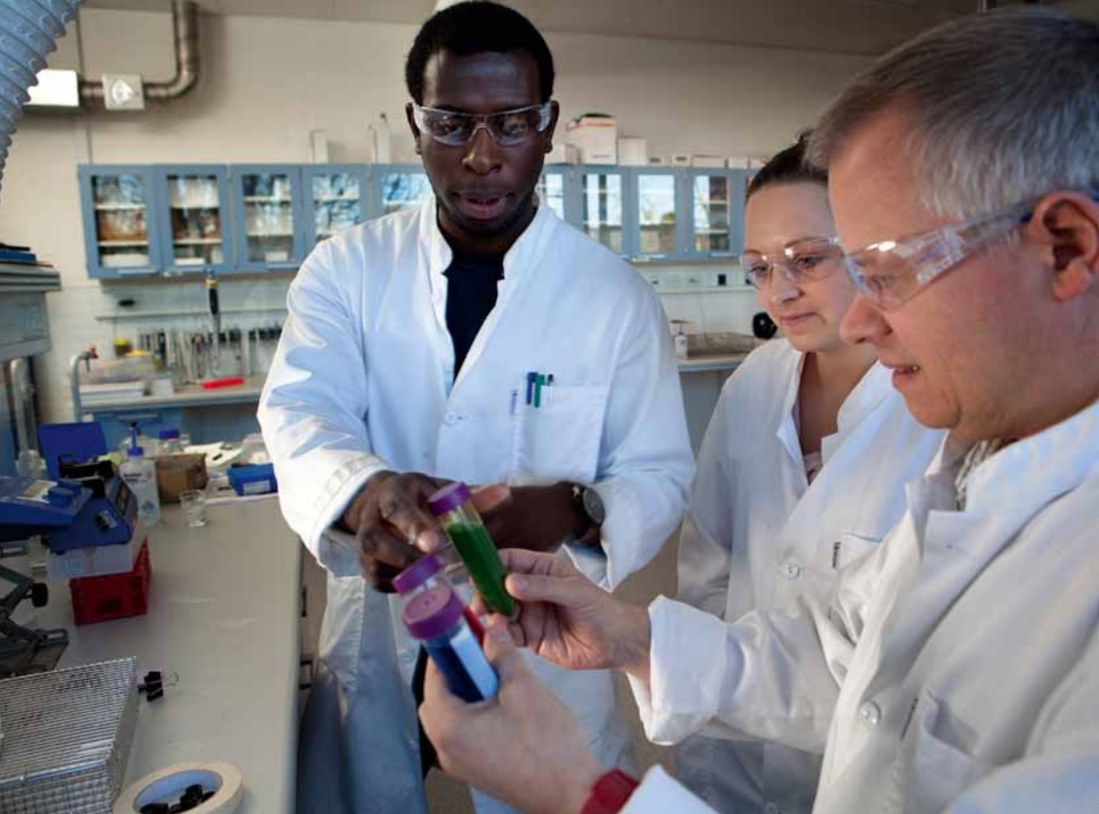
Multiphase reaction media (using dyed organic or aqueous phases for visual studies) is a feature of many of the new biocatalytic systems.
