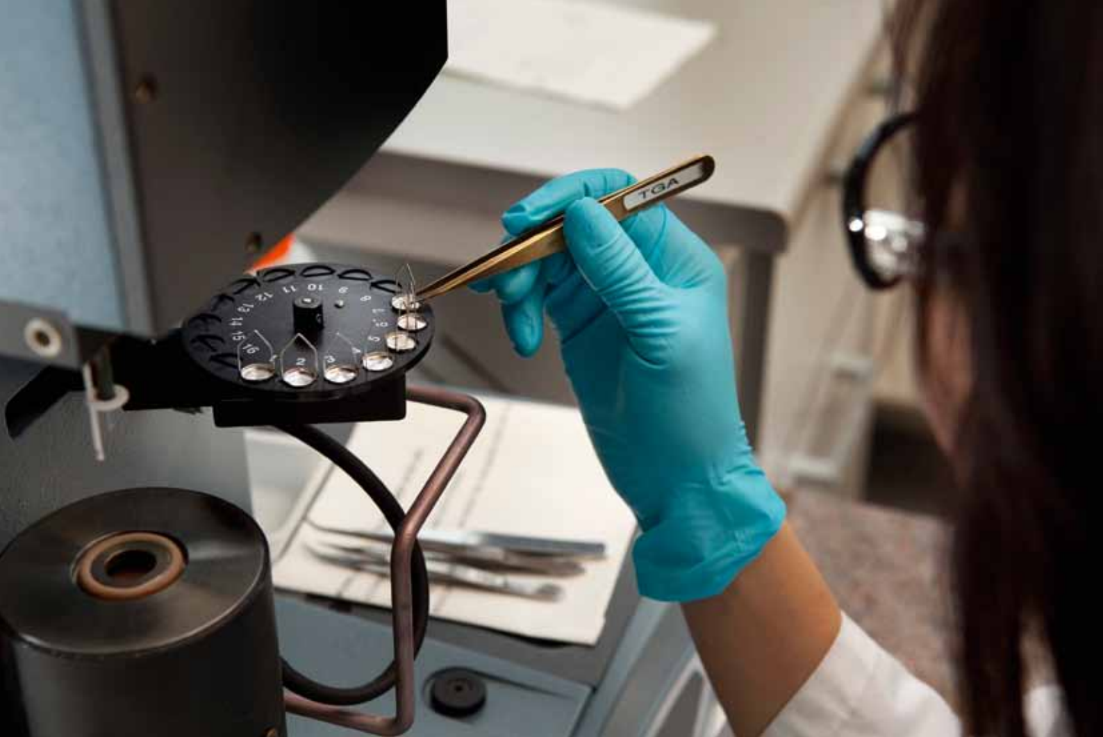
Kim Chi Szabo is loading the autosampler of the TGA Instrument with 7 polymer membranes in order to investigate the amount of surface grafted conducting polymer, and its influence on their thermal stability.
