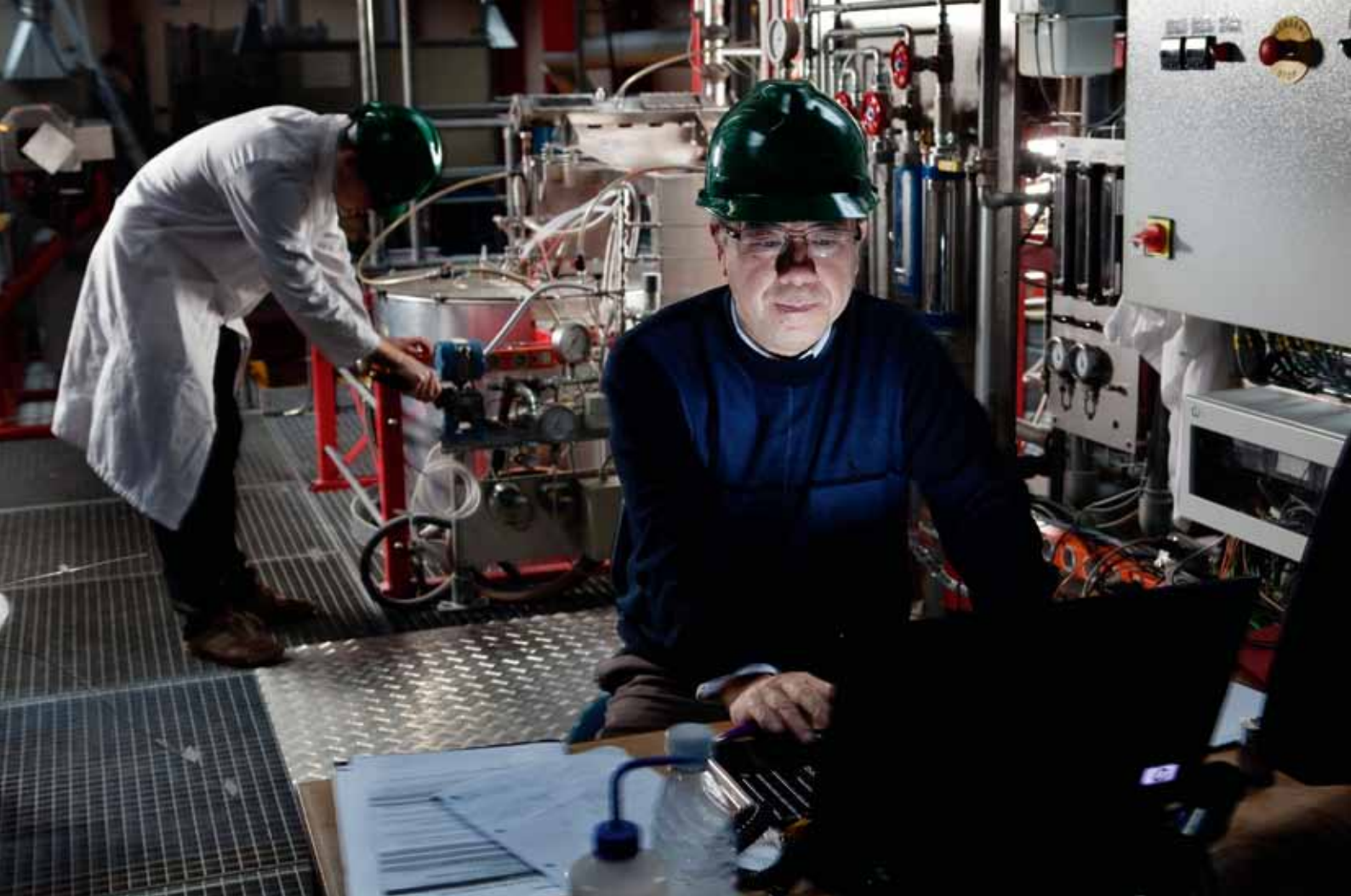
Associate Professor Weigang Li operating a pilot-scale swirl burner to co-fire pet-coke and sewage sludge for the cement industry.
