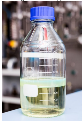
Figure 2: Photograph of recovered liquid from Exp. #4, oil is the top phase and the aqueous phase is the bottom phase in the bottle.
