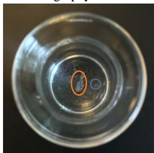
Figure 2: Photograph of separate crystals formed from crystallising product (highlighted in blue) in the presence of an externally added substrate crystal (circled in red).
