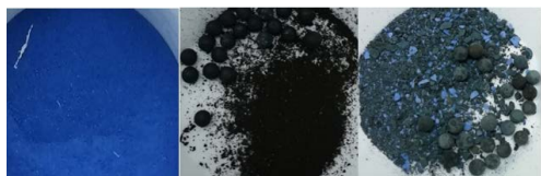
Figure 37: The appearance of the catalysts after (Left) co-impregnation, (Middle) impregnation with tin first, and (Right) impregnation with cobalt first.
