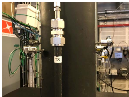
Figure 16. The optical sensors installed on the chimney of the wood stove setup
