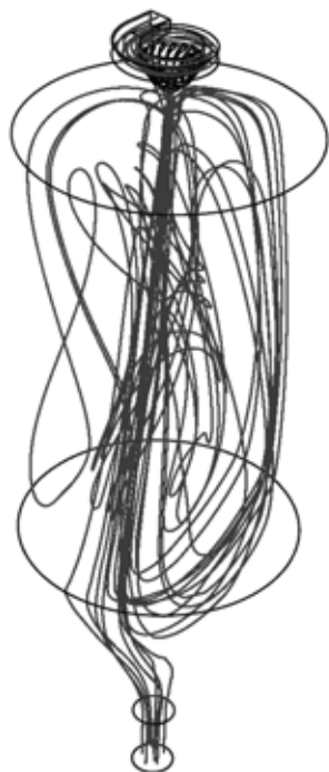
Figure 7: CFD-simulations of the air flow field inside the Novozymes spray dryer.
