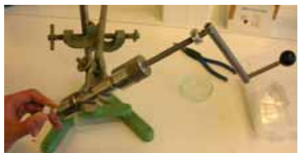
Fig.3 Extrusion device for block copolymer alignment
