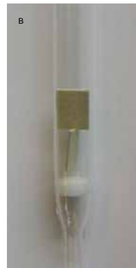
Figure 1: The lab-scale reactor (A). It consists in a quartz tube (B) with a quartz porous plate (5) for supporting the catalyst both as plates and powders. The whole reactor presents two different inlets (1 and 2) which allow keeping the reactants separated while heating to the reaction temperature, avoiding possible side reactions. The temperature in the reacting zone (6) is measured by a thermocouple inserted into (3). The gas finally exits the reactor from (4) and is then analyzed in composition.
