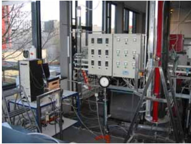
Figure 2: Experimental setup. To the left the SMPS system is placed and to the right the tubular furnace is seen.
