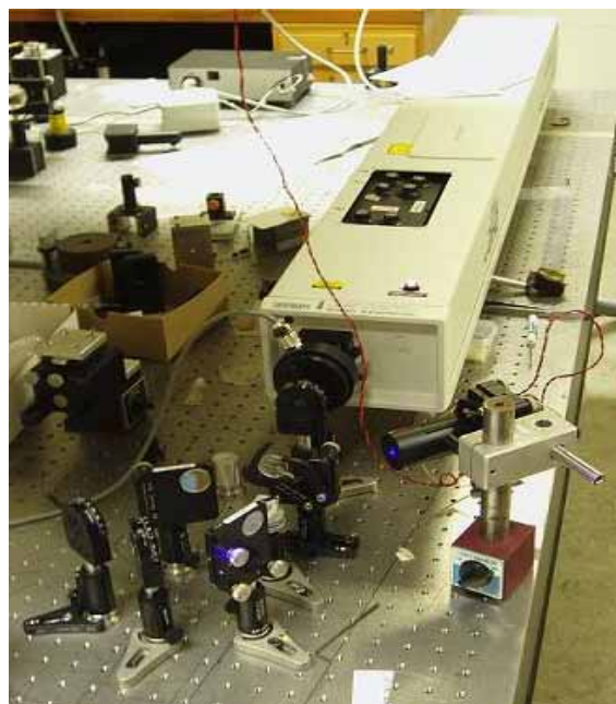
Figure 4a: The UV-laser setup, during an experiment on a uracil ornithine hexamer.
